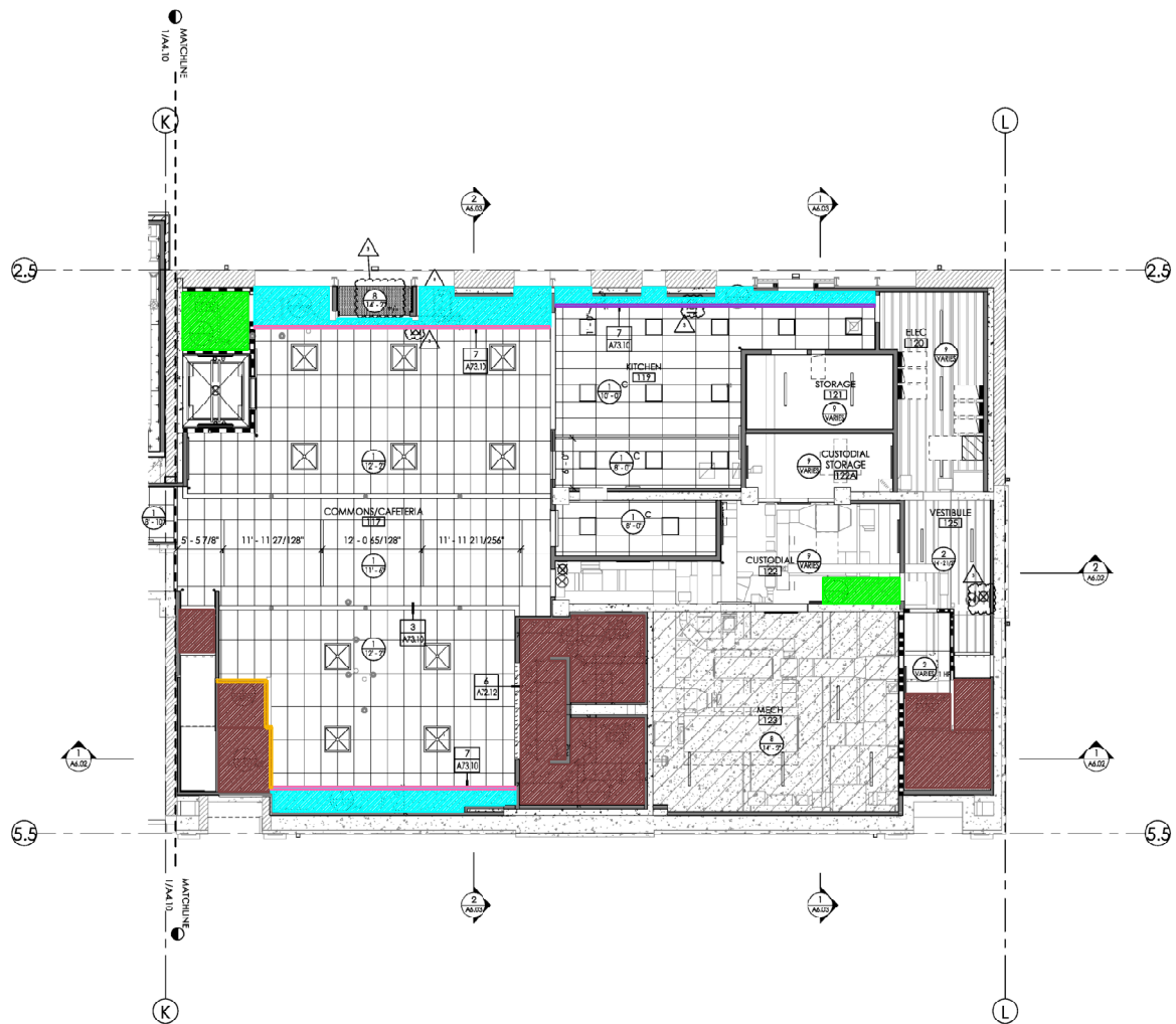
1 FIRST FLOOR REFLECTED CEILING PLAN - AREA 'B' 1/8" = 1'-0"
